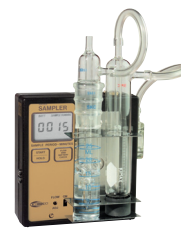
Impinger holder on pump with impinger and trap
