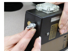
Thread exhaust port fitting into air discharge port on pump.
