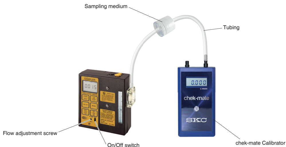
Figure 2. Calibration Train with Filter Cassette
