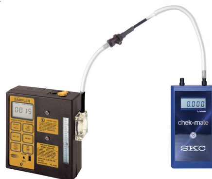
Calibration train with tube in low flow tube holder
