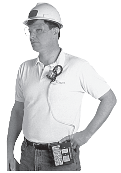
Clip sample medium to worker and pump to belt.
