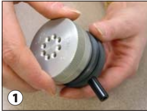
Unscrew impactor inlet from exhaust.
