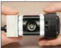
Correct: Eccentric centered in yoke
