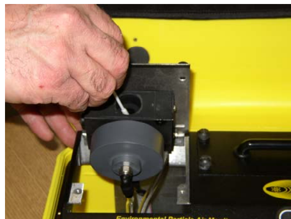
Figure 5-8. Sensor head being cleaned with cotton swab.
