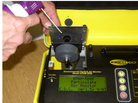
Figure 5-6. Dust being removed with low pressure air.
