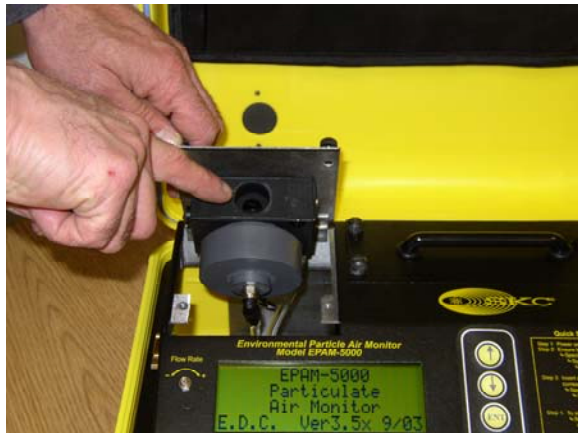
Figure 5-5. Removing the sensor covers. One cover located in front as shown in picture, the other cover is located on the right side of sensor not shown.
