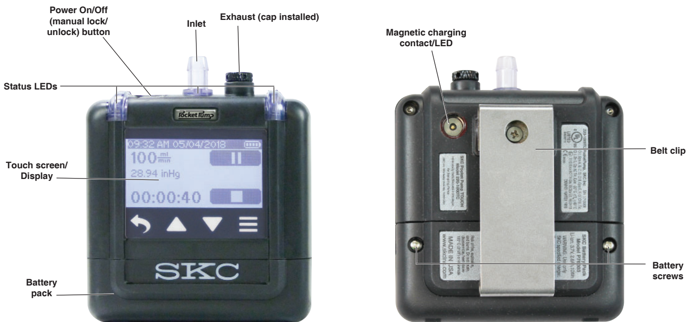
Figure 1. Pocket Pump TOUCH Physical Feature Overview
