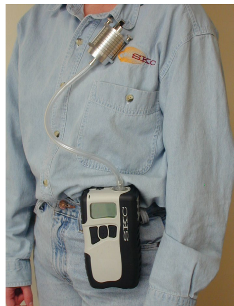
Sioutas Personal Cascade Impactor in Sampling Train
