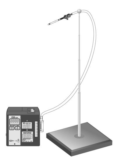
Figure 2. Portable area sampling system for solid adsorbent traps
