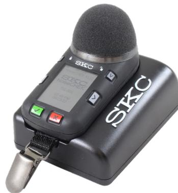
Secure magnetic charging dock available in 1 or 5-unit models. Provides USB connection to PC for use with DataTrac dB Software.
