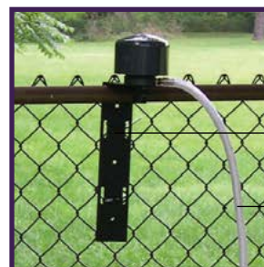
Rain cover protects sampling head
