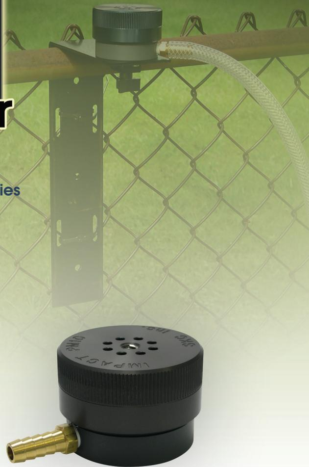
The patented\* SKC IMPACT single-stage inertial impactor is designed for efficient collection of PM10, PM2.5, or PM Coarse (10-2.5) in ambient air. Operated at 10 L/min constant flow, larger particles are captured on a disposable pre-oiled impaction disc while smaller particles collect on a 47-mm filter. The filter and impaction disc are housed in a removable filter cassette. The IMPACT's higher flow rate provides increased sensitivity for low levels of PM.
