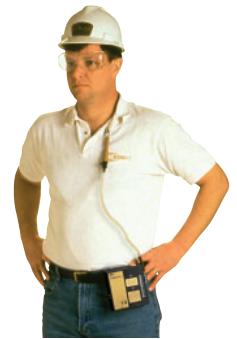
Clip holder to worker and pump to belt.
