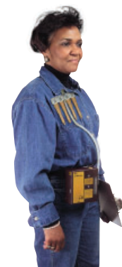
Clip holder to worker and pump to belt.
