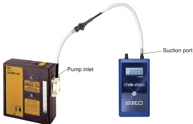
Flow rate verification train with tube in adjustable tube holder
