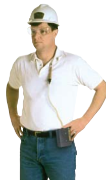
Clip tube holder to worker and pump to belt.
