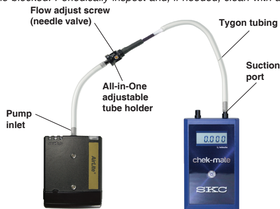
Calibration train with All-in-One connected to pump
