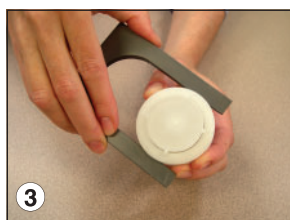
3a. Use the filter cassette opener to open filter cassette.
