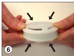
Press filter cassette top into filter cassette bottom.
