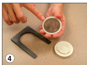
Ensure the stainless steel support screen is in place in the bottom of the filter cassette.
