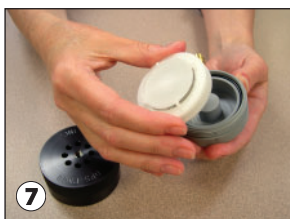
Reinsert cassette into impactor.
