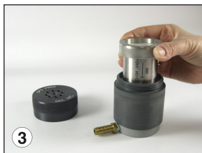
Insert media cartridge into cartridge holder section.
