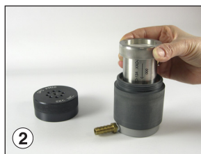
Lift media cartridge from cartridge holder section.
