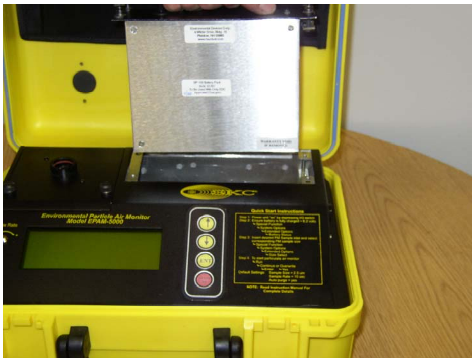
Figure 5-3. Diagram of battery being removed from EPAM-5000.
