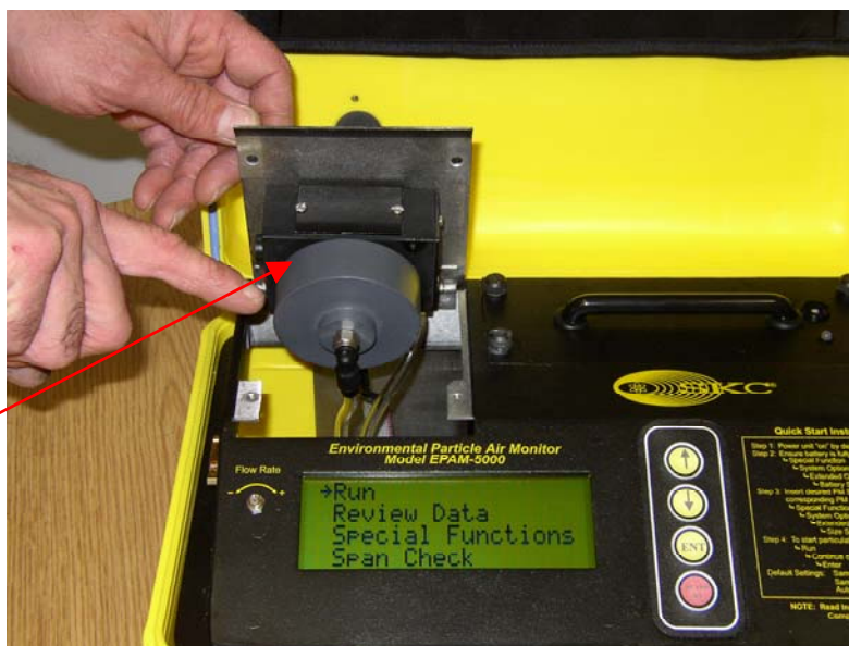
Figure 3-2. Diagram of sensor lid. To unlock sensor lid unscrew potted screw located on right side of sensor lid to expose the filter cassette. *NOTE: When closing sensor cover be sure not to tighten potted screw too tightly the spring inside the screw can break.
