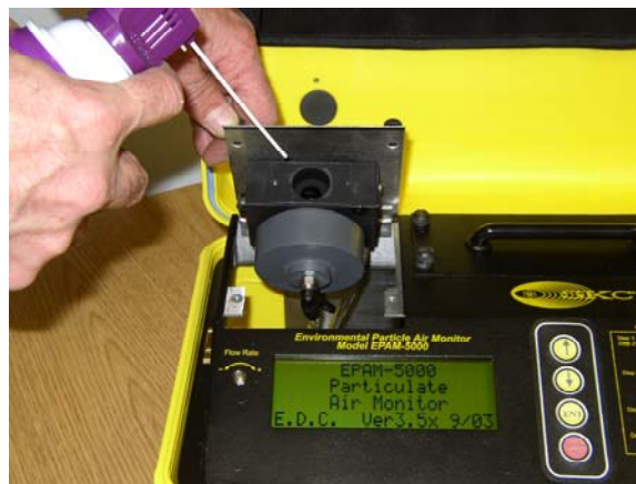
Figure 5-6. Dust being removed with low pressure air.
