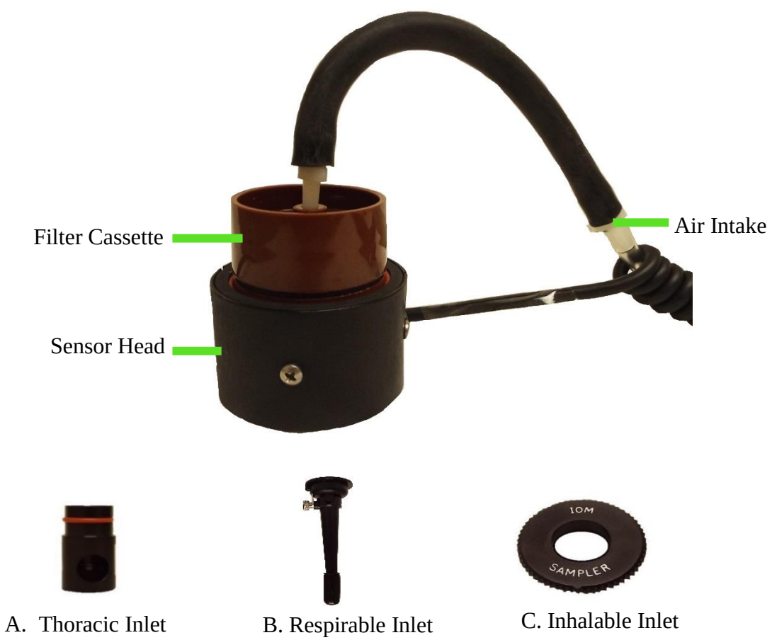
Figure 3-2. Diagram of sampling inlets for Thoracic, Respirable, and Inhalable. Pictures are not to scale.
