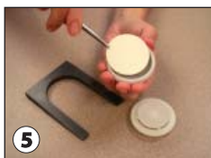
5 Using forceps accessory, place a preweighed 47-mm filter on the support screen.
