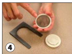
4 Ensure the stainless steel support screen is in place in bottom of filter cassette.
