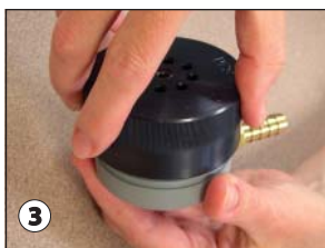
Place filter cassette on exhaust and screw impactor inlet and exhaust together just until tight. Further hand-tighten by 1/4 turn only.
