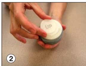
Place impaction disc on filter cassette top. The rough side of the impaction disc should face up. SKC-supplied discs are stamped with "UP" on the appropriate side.
