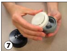
Reinsert cassette into impactor.
