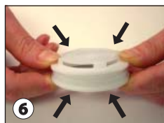
6 Press filter cassette top into filter cassette bottom.
