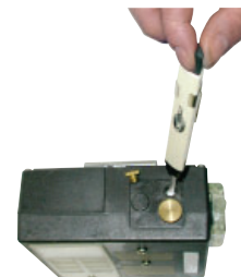
For low flow, turn regulator valve screw counterclockwise.
