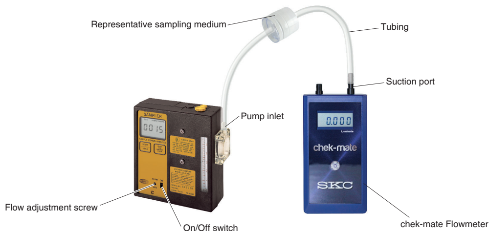
Figure 2. Flow Rate Verification Train with Filter Cassette
