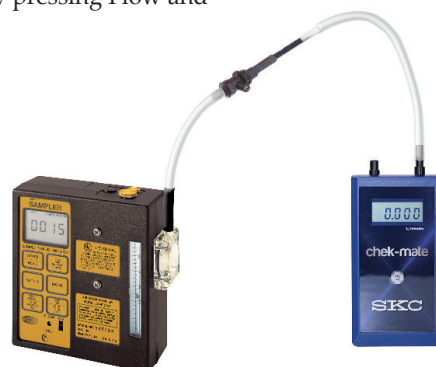
Flow rate verification train with tube in low flow tube holder
