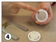
4 Ensure the stainless steel support screen is in place in the bottom of filter cassette.
