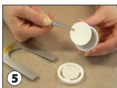
5 Using the forceps accessory, place a preweighed 37-mm filter on the support screen.
