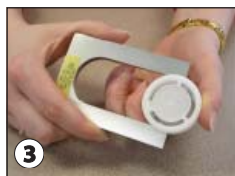
3 Use the cassette opener accessory to open filter cassette.
