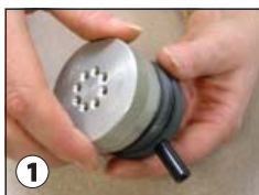
1 Unscrew inlet from exhaust.
