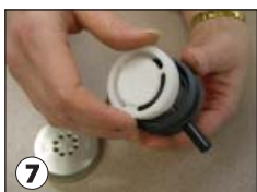
7 Reinsert cassette into impactor.
