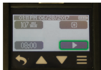
> Touch Time button in Flow Menu to set sample duration.
