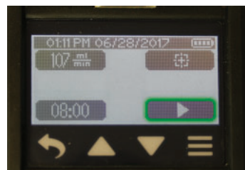
> Touch Run button in Flow Menu to run pump in constant flow.
