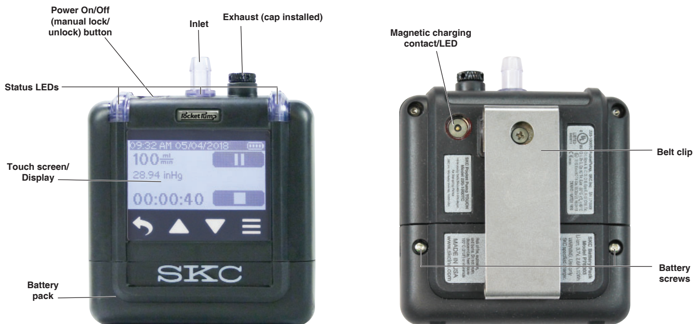
Figure 1. Pocket Pump TOUCH Physical Feature Overview
