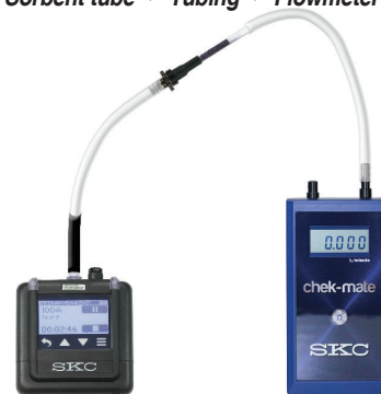
Figure 3. Single-tube Flow Rate Verification Train
