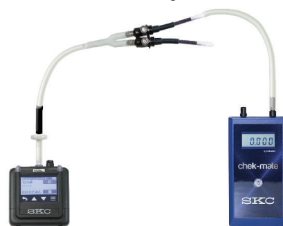
Figure 4. Multiple-tube Flow Rate Verification Train - Constant Flow
