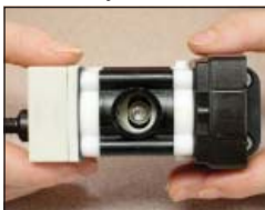
Correct: Eccentric centered in yoke
