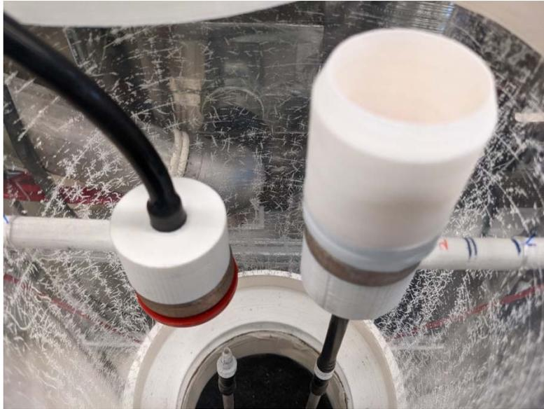
Picture 3. Location and orientation of PPI-8 L/min impactor in the test chamber when it was tested facing down. This test was performed with NaCl particles only.
