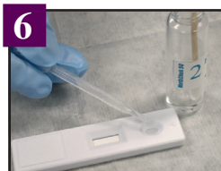
6 Pipette 3 drops vial liquid into "S" well on Step 3 Cartridge.
