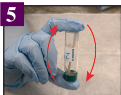
5 Extract Insert swab tip in Step 2 Extractor vial, break off swab, cap vial, and rotate slowly end-to-end.
