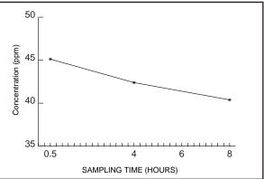
The mean sampling rate was 13.1 ml/min  $(3.29 \mu g/ppm/hr)$  and was calculated as the mean of all the exposure periods, based on a reference concentration of 42.6 ppm.
