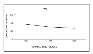
The mean sampling rate was 13.1 ml/min (3.27 µm/ppm/hr) and was calculated as the mean of all data based on a reference concentration of 40.5 ppm.
